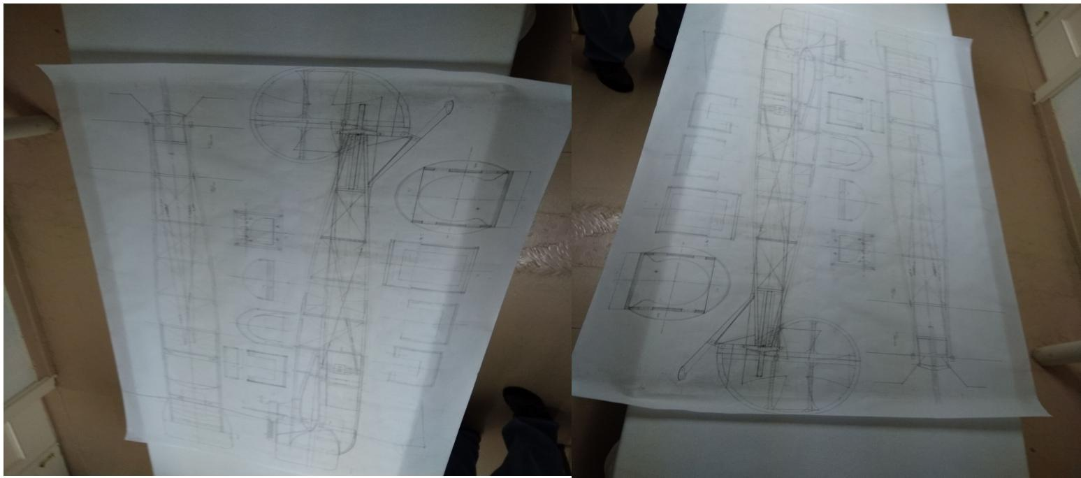
The plans I am drawing are for a stand off scale WW1 Fokker Eindecker. It will have a wingspan of 81 inches and powered by a .90 fs. Carbon fiber will be used to reinforce diagonally within the fuselage structure. Covering will be silk and dope, cowl will be molded fiberglass. Ailerons will be added in place of wing warping as in the full scale original.
